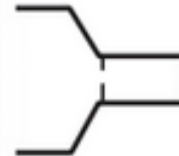
Slip Tip - slip or push-on connection.
